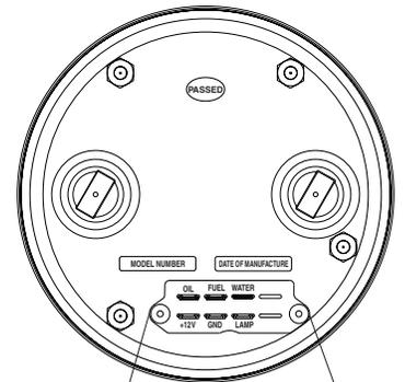
Install grounded wire to sender flange screw for proper operation
