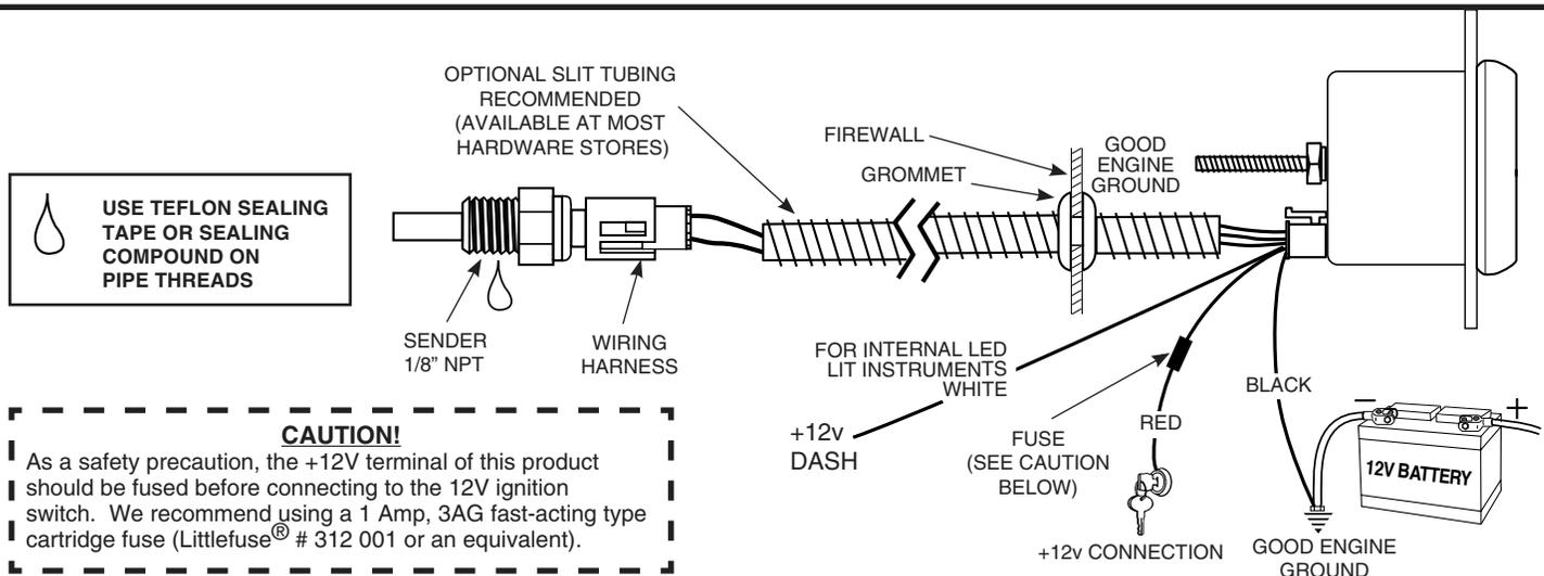
**USE TEFLON SEALING TAPE OR SEALING COMPOUND ON PIPE THREADS**
