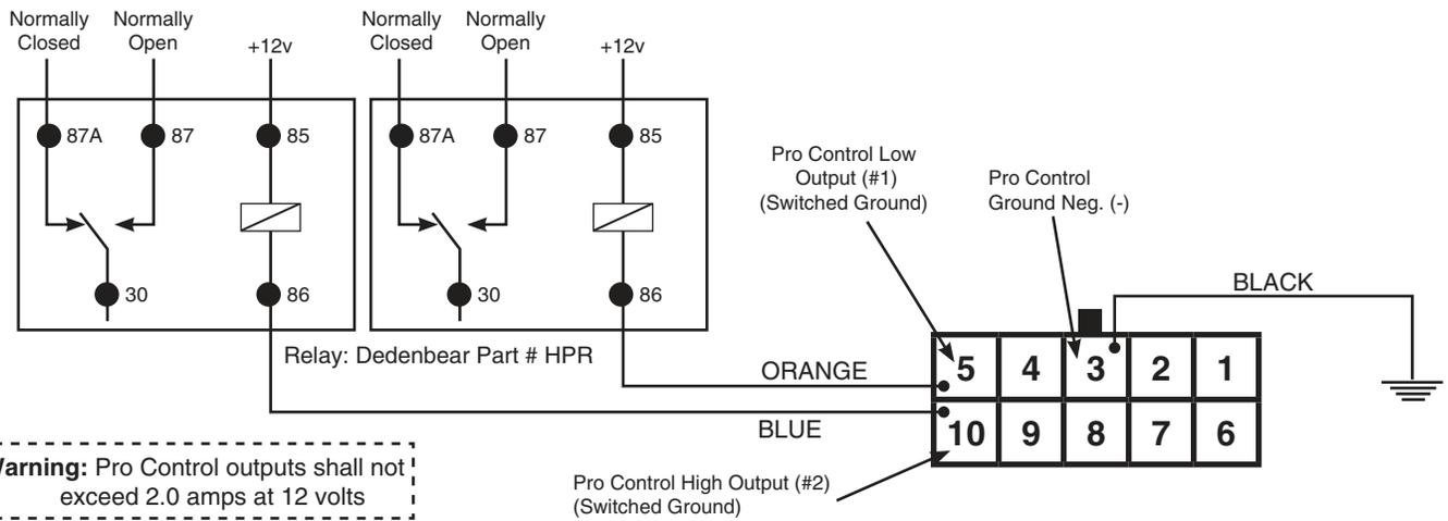
**Warning:** Pro Control outputs shall not exceed 2.0 amps at 12 volts
