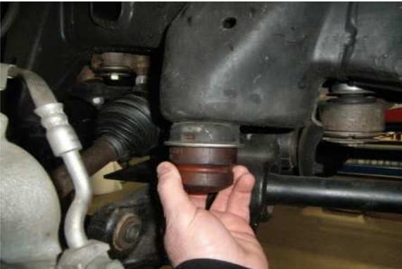
Remove factory lower control arm bump stops (4)
