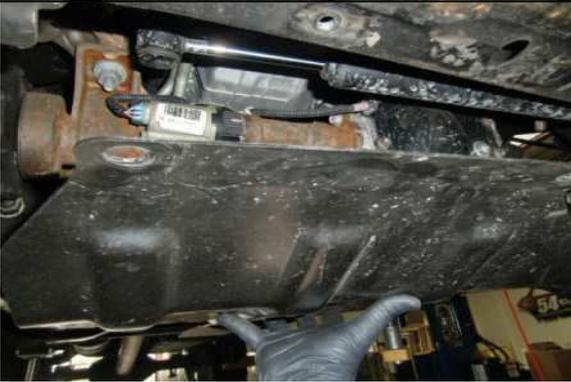
Remove skid plate bolts and skid plate
