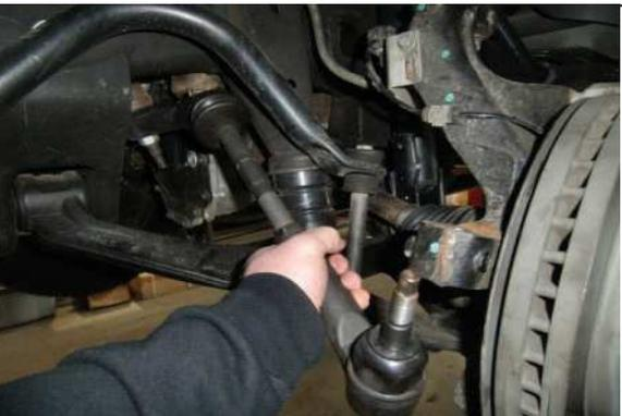
Install new steering assembly on center link
