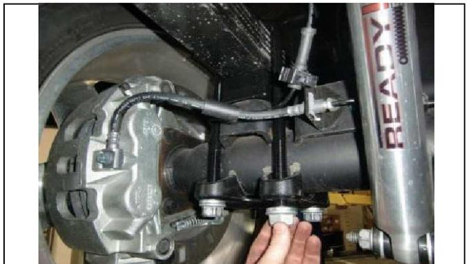
Install new longer u-bolts and install new hardware,
