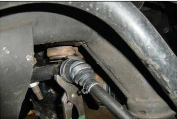
Loosed and remove inner/outer tie rod from center link.
