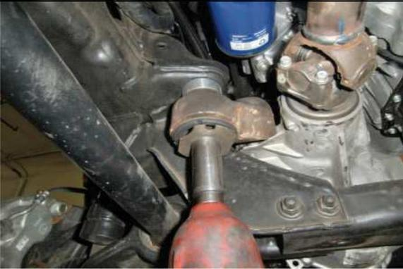
Install (4) differential drop spacers with new hardware
